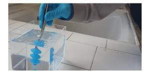
The use of tweezers allows the printed parts to be removed from the gel carrier without damage.
