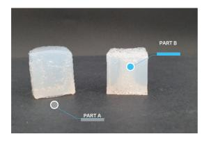
Gel back pressure changes the shape of the liquid bead by increasing its length on Z-axis while reducing it on X and Y axes. For a cube with a volume of 20 mm, a deformation of 3 mm on the Z axis can be observed (A).
