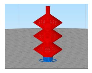
Silicone 3D printing with support gel requires the use of a slicer (slicing software) allowing multiprocessing.
