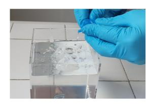
Hollow parts might trap some gel. Therefore, we recommend including, when designing the part, a feature that allows the gel to drain away. In this manner, you will be able to purge it once the part is cured.
