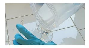
Air bubbles generated by pouring may alter quality of part (entrapped bubbles, holes). Be sure to pour the product gently to avoid any defects in the part. Replace the support gel when loaded with bubbles, while pouring or after printing.
