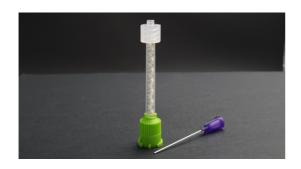
RTV-2 silicone 3D printing in the support gel requires the use of a Luer lock type needle. Adapt needle length to the container height. The needle used for the accordion measures 34 mm.
